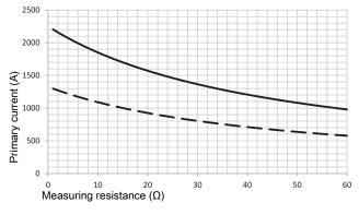
$\begin{array}{c} ---- U_{C} = \pm 24 \ V \ -5 \ \%, \ T_{A} = 85 \ ^{\circ}C \\ ---- U_{C} = \pm 15 \ V \ -5 \ \%, \ T_{A} = 85 \ ^{\circ}C \\ Primary currents higher than I_{PM} only for peak! \end{array}$
